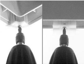
Place over the screw holes on the inside of the frame, the 8 fixing brackets; four in each corner, four in the centre of each side. Secure with screws, stop as soon as the brackets start to distort.
