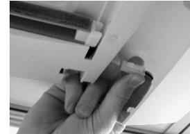
Fix the connector from the inner frame with the connector from the side panel before inserting the side cover.
