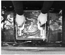
Clean the gaps by immersing the hood in a container filled with water. Let the dirt soak a little. Use the two handles to pull the hood through the water so that the dirt can be washed out.
