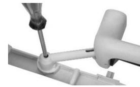
For easier cleaning of the dome it can be removed from the frame by releasing the four screws holding the handle arms.
